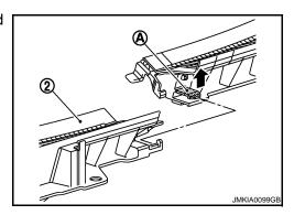
8. Plastic pawl (B) is push down and cowl top cover LH (1) is removed ahead of vehicles.
