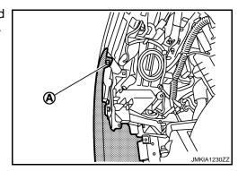
8. Pull the bumper fascia side toward the vehicle side to disengage the fitting of bumper side bracket and bumper fascia side.
