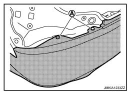
4. Remove bolts (A) of bumper fascia underside (LH/RH).
