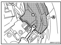
5. Remove bolts (A), and then remove bumper bracket (1).
