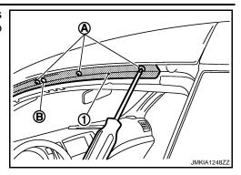
4. Remove front pillar finisher (1) fixing clips with remover tool (A).
