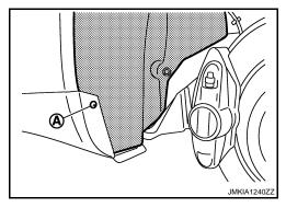
3. Remove rear wheel house protector mounting nuts and then remove rear wheel house protector.
