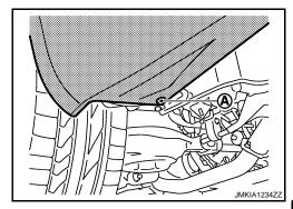
Remove screws (A) of bumper fascia front end upper (LH/RH).
