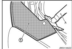
4. Disengage trunk drip cover (1) fixing metal clip using remover tool (A).
